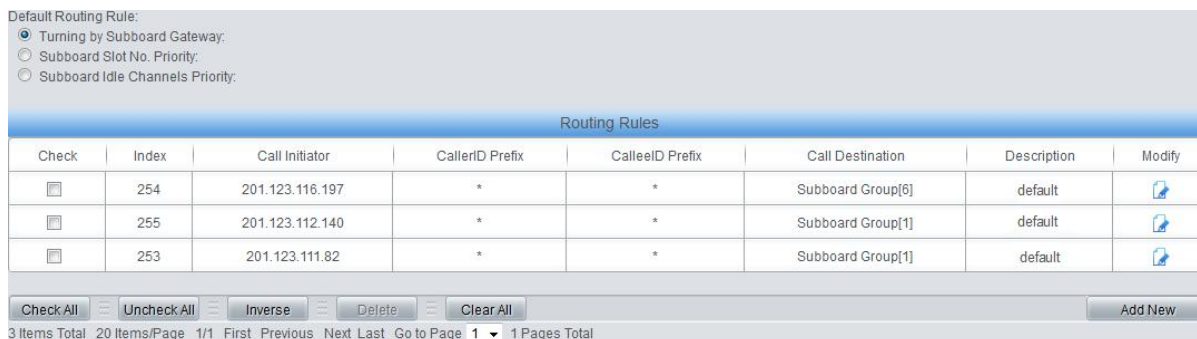
Figure 3- 14 IP→TEL/PSTN Routing Rule Configuration Interface
