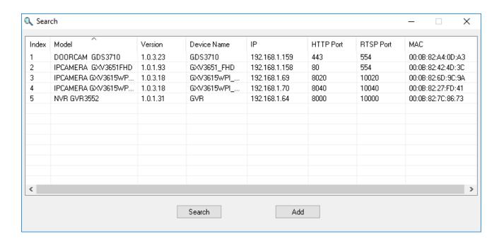
4. Double click the selected product (like DOORCAM GDS3710) will trigger the default browser to running with the displayed IP as URL. User can then configure the device through the webGUI after entering the correct credentials.
